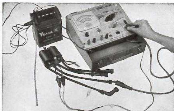
Fig. 7-8 Ignition coil test
