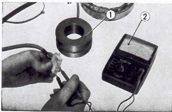
Fig. 8-8 ① Field coil ② Tester
